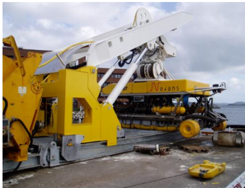
Figure 5. CapJet 1 MW ready for deployment with its launch and recovery system.
